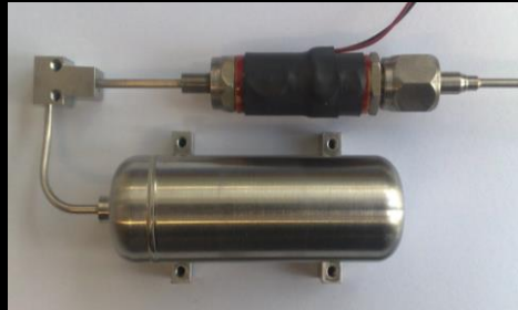
Miniature gas valve and Calibration gas system
